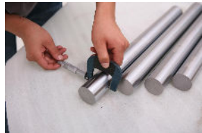
Piston rod outer diameter detection
